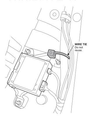
Remove the three XM unit bracket nuts.
