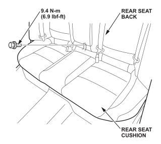
2. While pushing down on the seat cushion, pull the seat hook handles to release the hooks.
