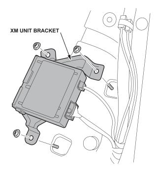
7. Slide the transceiver onto the bracket.
